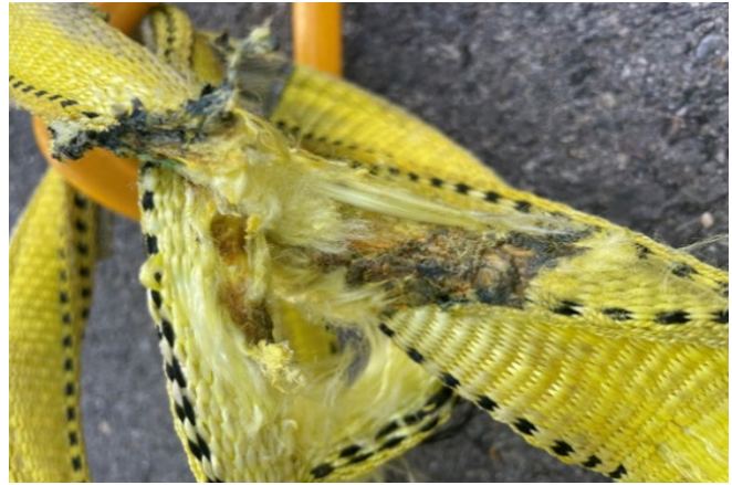
Melted Liftex Strap near Gunnebo Shackle
