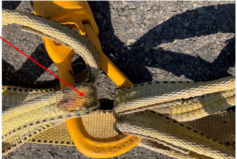
Faded areas, showing UV damage to straps
