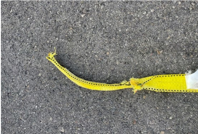
Broken Liftex Strap
