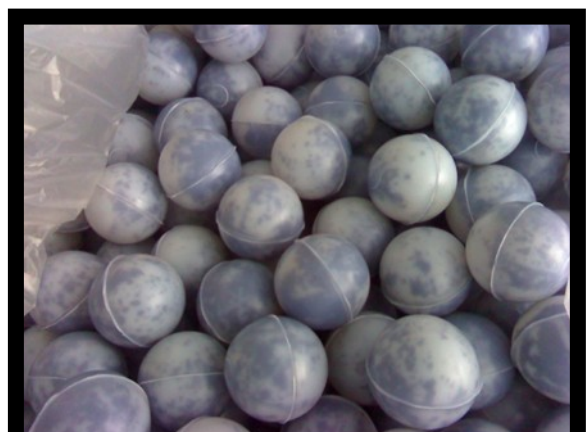
Figure 1. VPL's Premo plastic spheres with excess plastic around the seam.
