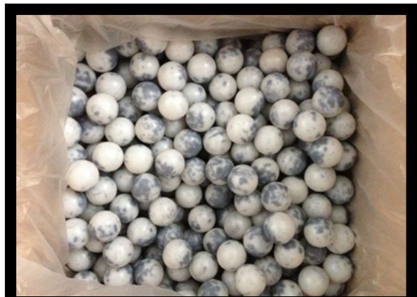
Figure 2. SEI's Premo spheres with a spotted appearance on the internal surface. Some of VPL's Premo spheres also have a spotted appearance (figure 1).
